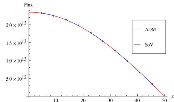
Figure 2 – Neutron flux for  $y=0$ .
